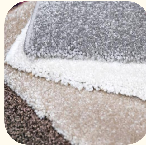
Cut Pile (1-pile height)
